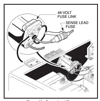
Figure 26 Sense Lead Fuse
