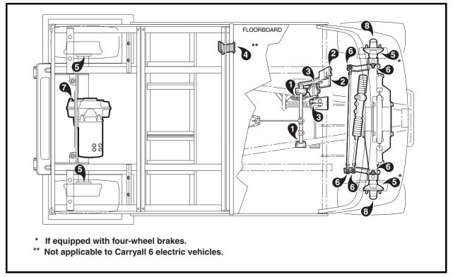
Figure 21 Lubrication Points – Electric Vehicles
