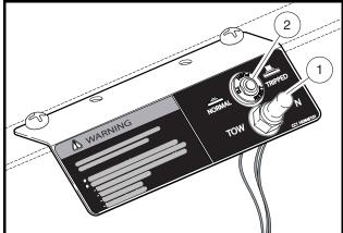
Figure 11 Tow/Run Switch - IQ System
