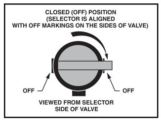
Figure 18 Fuel Shut-off Valve - Closed Position
