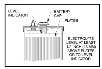
Figure 23 Electric Battery Electrolyte Level
