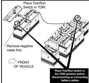
Figure 4 Carryall 6 IQ Plus Electric Vehicle
