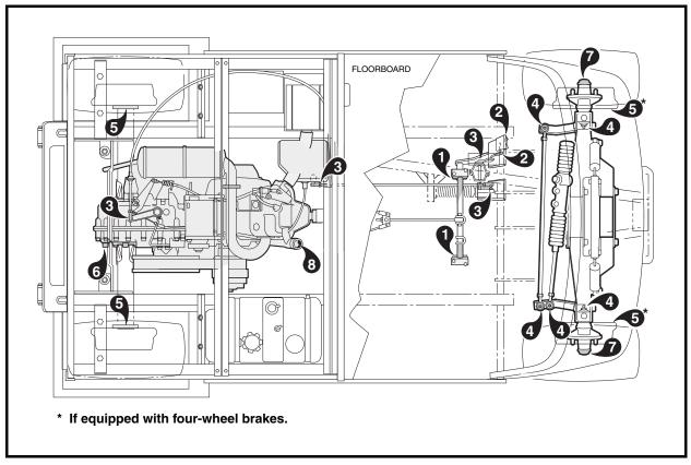
Figure 22 Lubrication Points – Gasoline Vehicles
