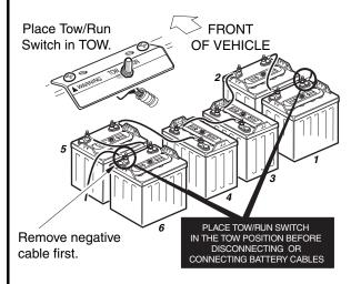
Figure 1 Gasoline Vehicle
