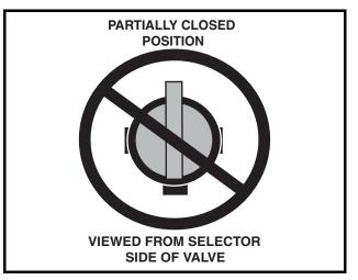
Figure 20 Fuel Shut-off Valve – Partially Closed Position
