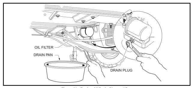
Figure 29 Engine Oil Drain Plug and Pan
