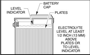
Figure 28 Gasoline Battery Electrolyte Level
