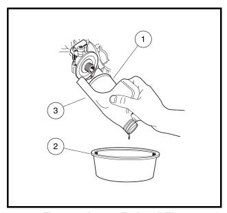
Figure 30 Remove Engine Oil Filter
