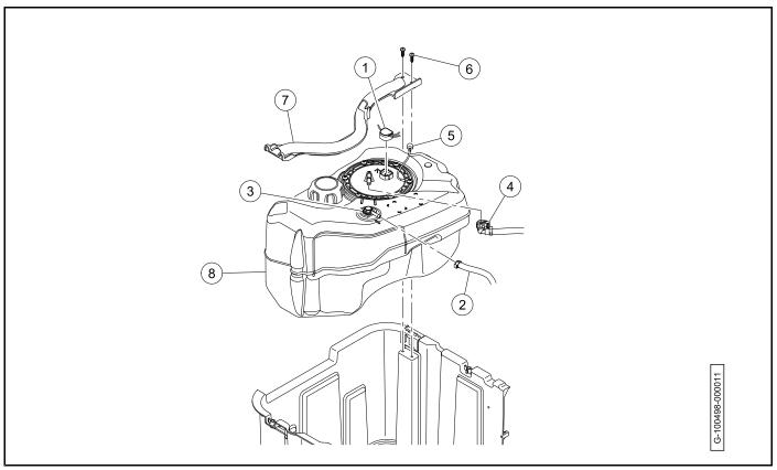
Figure 21-22 Fuel Tank Installation
