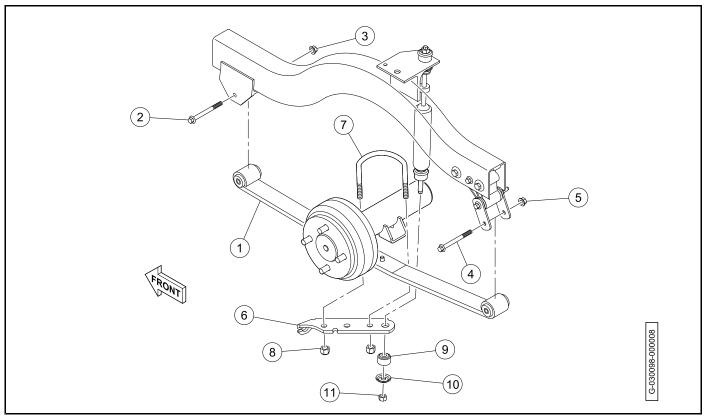
Figure 9-7 Leaf Spring Installation - Two-Passenger
