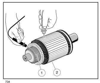
Figure 16-12 Armature Test
