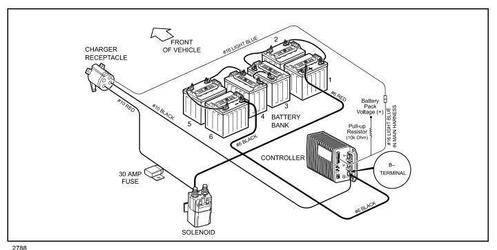
Figure 15-6 Charge Circuit – External High-Frequency Charger
