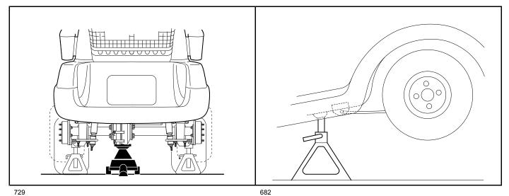
Figure 16-1 Lift Vehicle with Floor Jack
