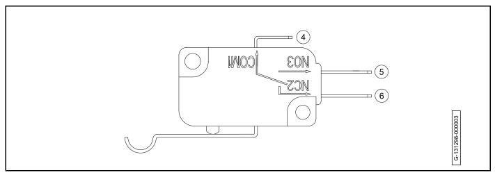
Figure 19-28 Neutral Lockout Limit Switch Terminals
