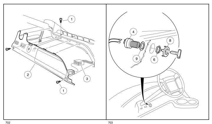
Figure 13-1 Instrument Panel Removal
