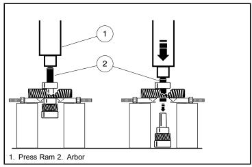
Figure 17-12 Intermediate Gear Assembly
