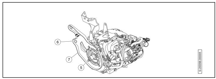
Figure 20-2 Clutch Plate Removal
