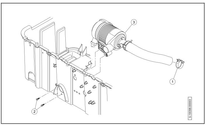
Figure 21-10 Air Intake System
