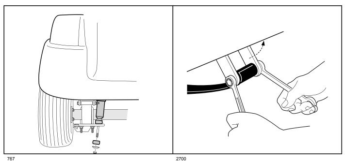
Figure 17-8 Disconnect Shocks
