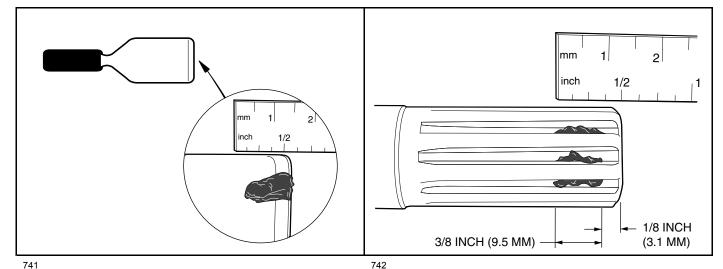
Figure 16-20 Grease on Putty Knife
