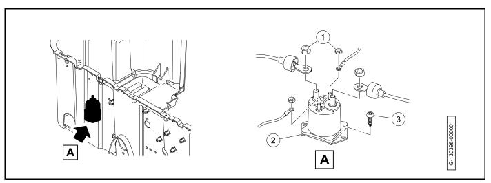
Figure 19-18 Solenoid Removal
