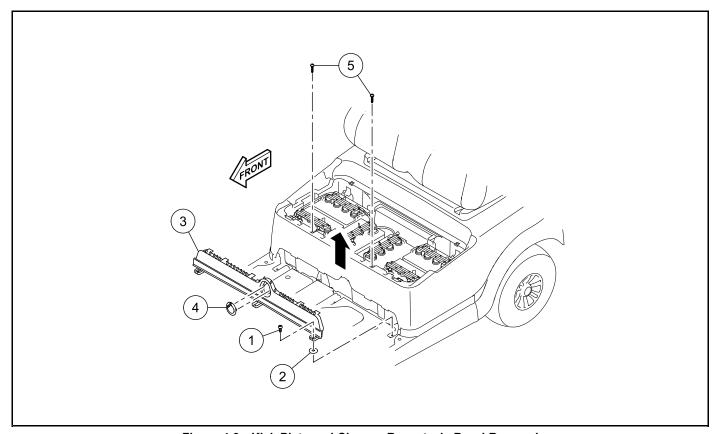
Figure 4-9 Kick Plate and Charger Receptacle Bezel Removal
