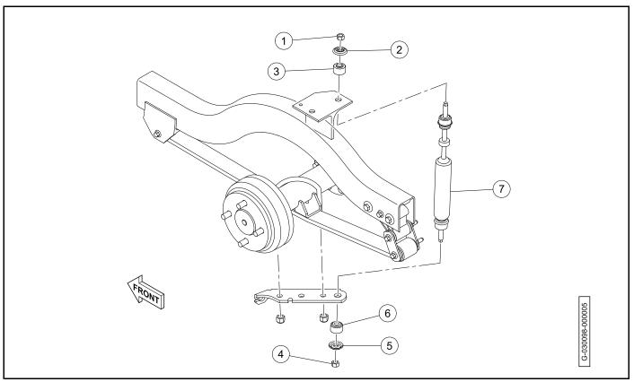
Figure 9-2 Rear Shock Absorber Removal
