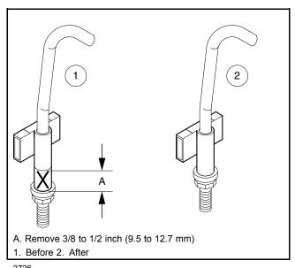
Figure 19-17 Belt Tension Tool Modification (If Necessary)
