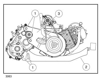
Figure 24-13 Transaxle Mounting Bolts
