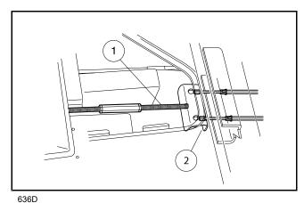
Figure 6-30 Install Cables In Equalizer Bracket
