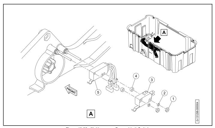
Figure 19-25 Multi-purpose Buzzer Limit Switch
