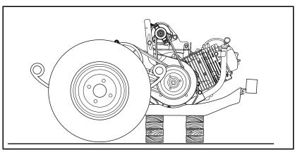
Figure 24-12 Remove Powertrain and Place Wood Blocks Under Engine Pan
