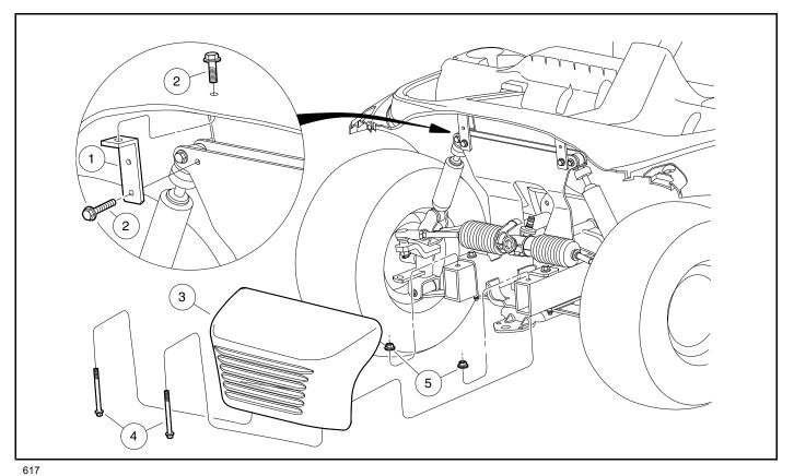
Figure 4-4 Bracket and Front Bumper
