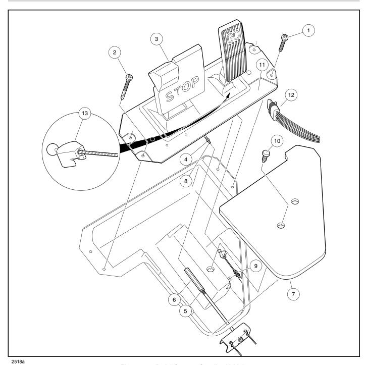
Figure 5-4 Pedal Group – Gasoline Vehicle
