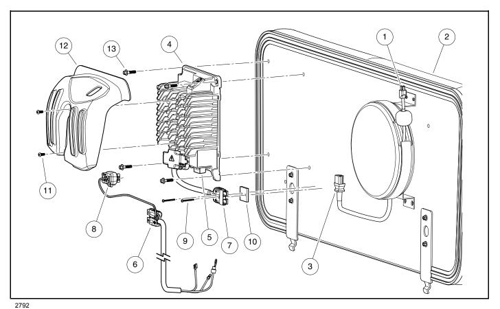
Figure 15-12 Onboard High-Frequency Charger Mounting
