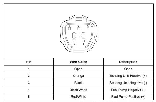
Figure 18-13 Fuel Pump Connector
