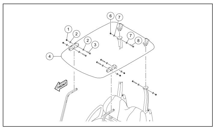
Figure 4-15 Two-Passenger Canopy Removal
