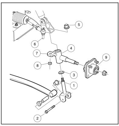
1312D Figure 7-18 Kingpin and Steering Spindle Installation
