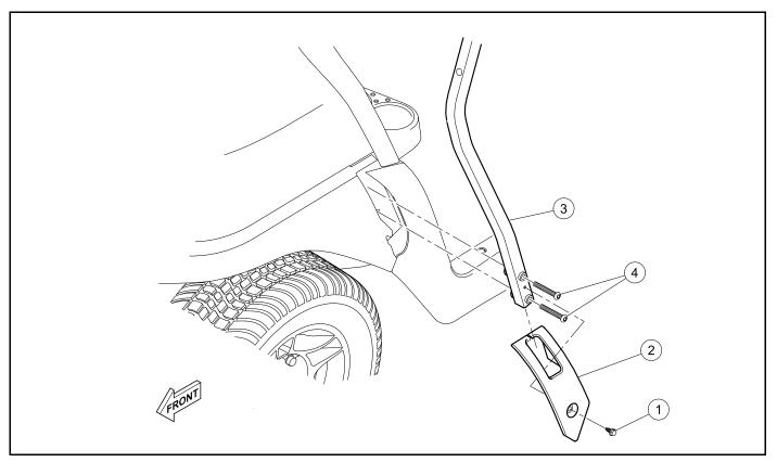
Figure 4-38 Front Canopy Strut Installation
