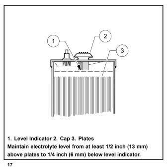
Figure 14-3 Battery Electrolyte Level
