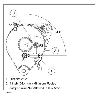
Figure 19-12 A1 to F1 Terminal Jumper Wire Routing
