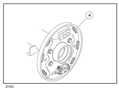
Figure 6-8 Apply Grease On Bosses
