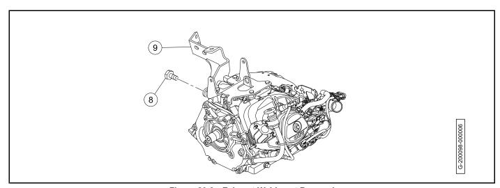
Figure 20-3 Exhaust Weldment Removal
