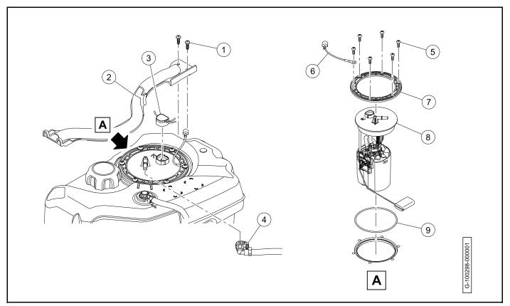
Figure 21-19 Fuel Pump Module Removal
