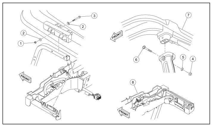
Figure 4-20 Two-Passenger Canopy With Display Unit Installation
