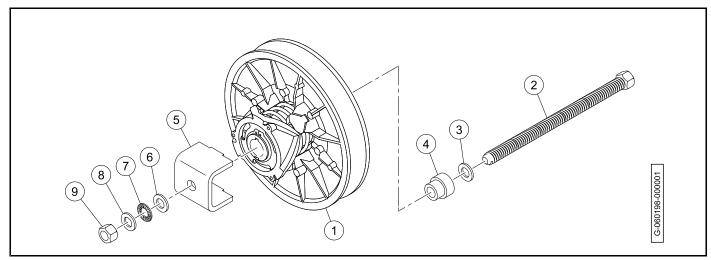
Figure 23-14 Driven Clutch Tool - Disassembly
