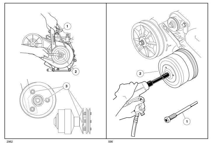
Figure 23-3 Loosen Retaining Bolt
