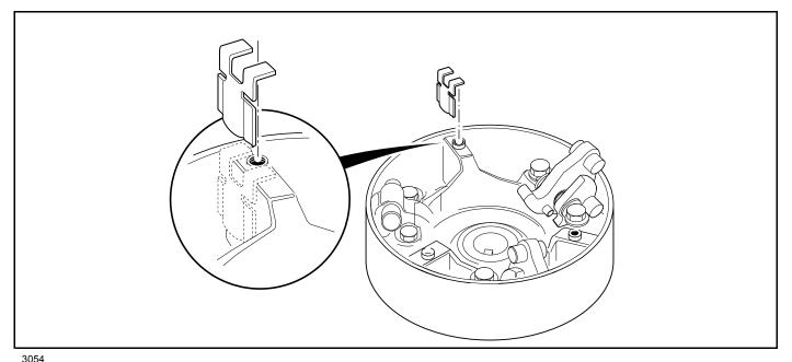
Figure 23-12 Correct Orientation of Drive Button Take-up Springs
