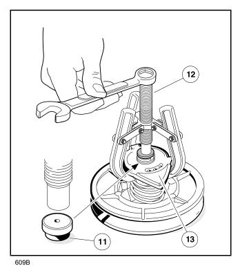
Figure 23-16 Cam Removal
