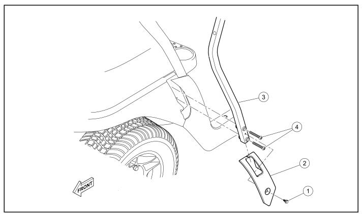
Figure 4-21 Front Canopy Strut Removal
