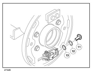
Figure 6-5 Remove Adjuster Wheel
