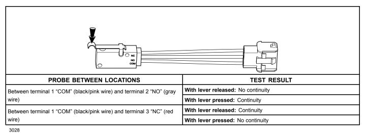
Figure 18-7 Transaxle Limit Switch Test
