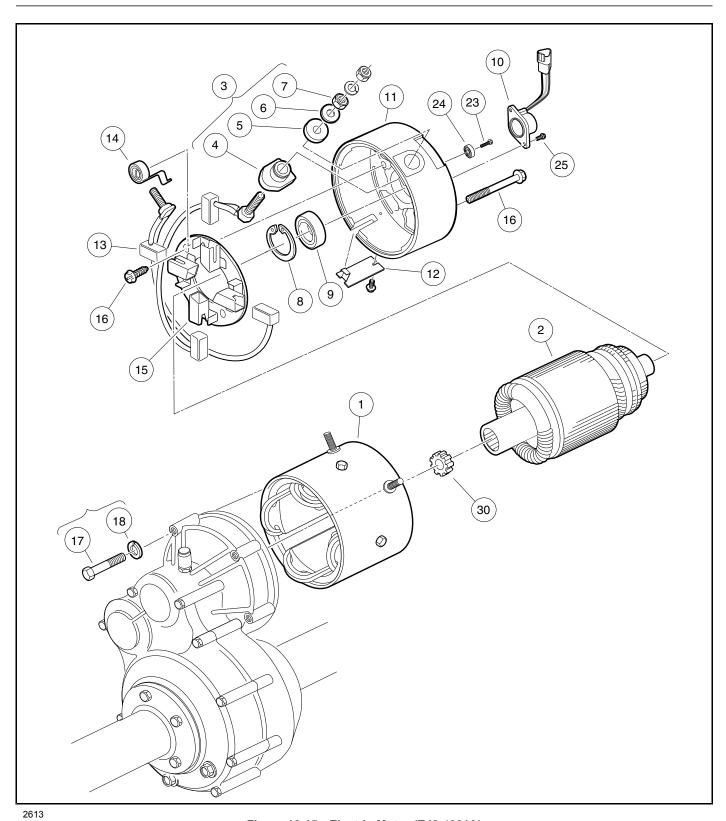
Figure 16-15 Electric Motor (EJ8-4001A)
