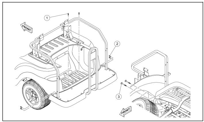
Figure 4-51 Foot Deck (2+2) Removal
