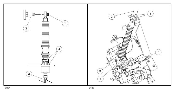
Figure 24-15 Shifter Cable at FNR Handle
