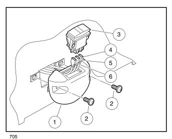
Figure 13-7 Forward/Reverse Rocker Switch
