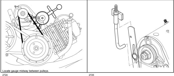
Figure 19-15 Belt Tension Gauge
