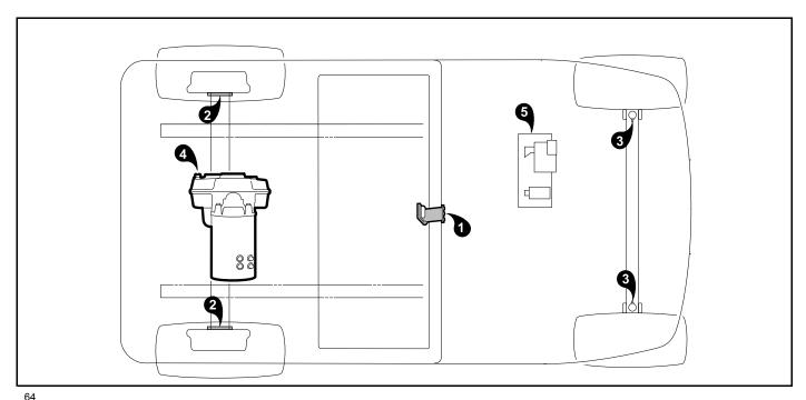
Figure 10-1 Lubrication Points – Electric Vehicles
