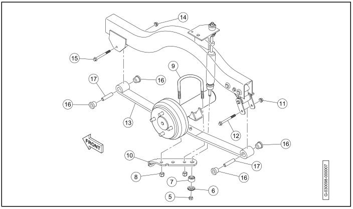
Figure 9-6 Leaf Spring Removal - Two-Passenger
