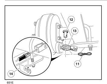
Figure 6-28 Disconnect Cables at Rear Brakes
