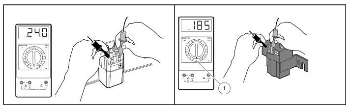
Figure 12-6 Activating Coil Test – Factory-installed Solenoid
