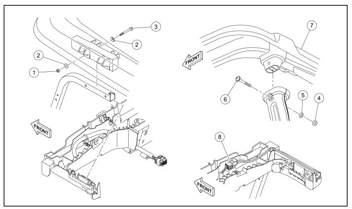
Figure 4-17 Two-Passenger Canopy With Visage Display Unit Removal
