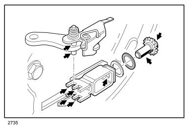
Figure 6-10 Apply Grease To Brake Adjuster
