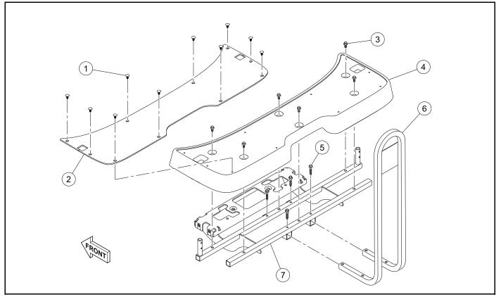
Figure 4-52 Foot Deck (2+2) Disassembly
