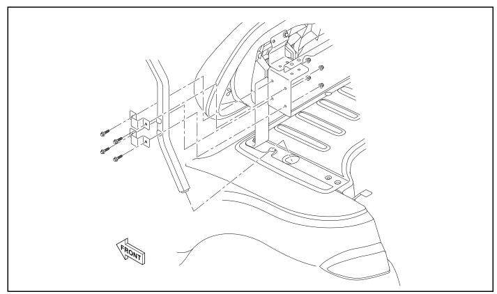
Figure 4-39 Rear Canopy Support Removal
