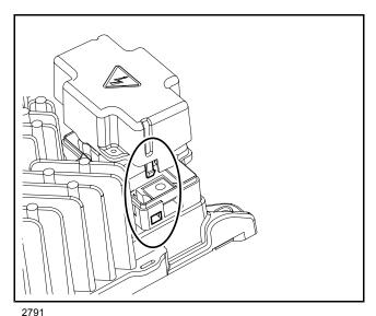
Figure 15-11 Terminal Block Cover Mounting Tabs
