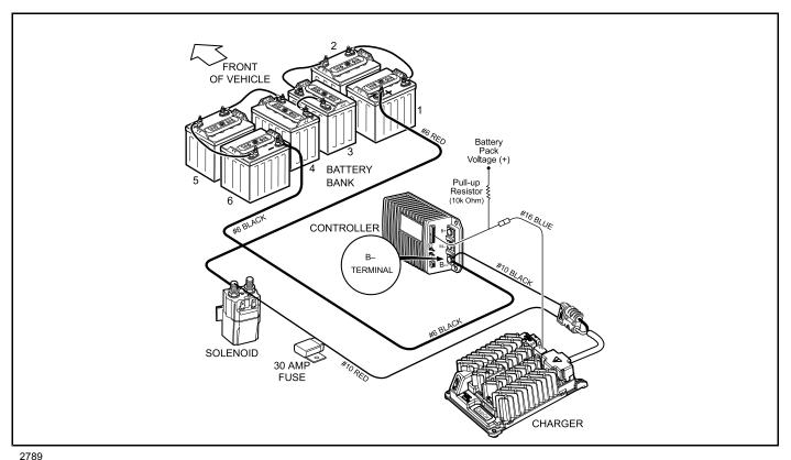
Figure 15-7 Charge Circuit – Onboard High-Frequency Charger
