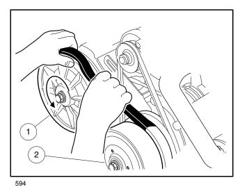
Figure 23-1 Drive Belt Removal
