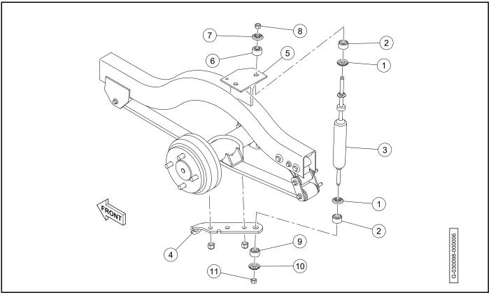
Figure 9-3 Rear Shock Absorber Installation
