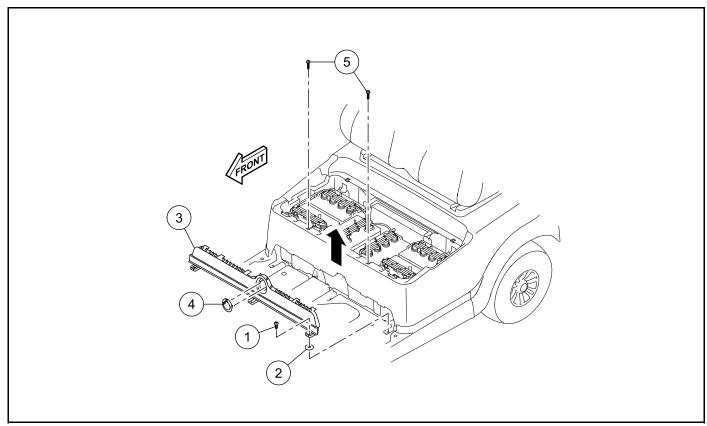
Figure 4-10 Kick Plate and Charger Receptacle Bezel Installation
