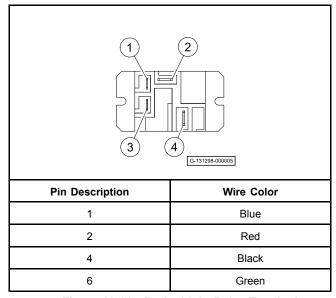
Figure 19-32 Brake Light Relay Terminals
