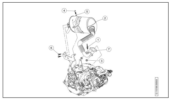
Figure 22-1 Muffler Removal
