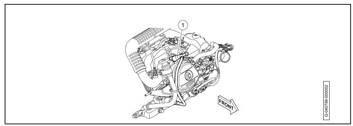
Figure 3-2 Spark Plug Wire
