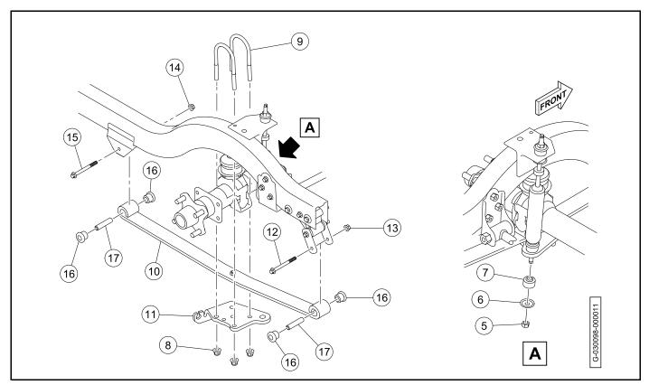
Figure 9-14 Leaf Spring Removal (Four-Passenger - Heavy Duty With Panhard)
