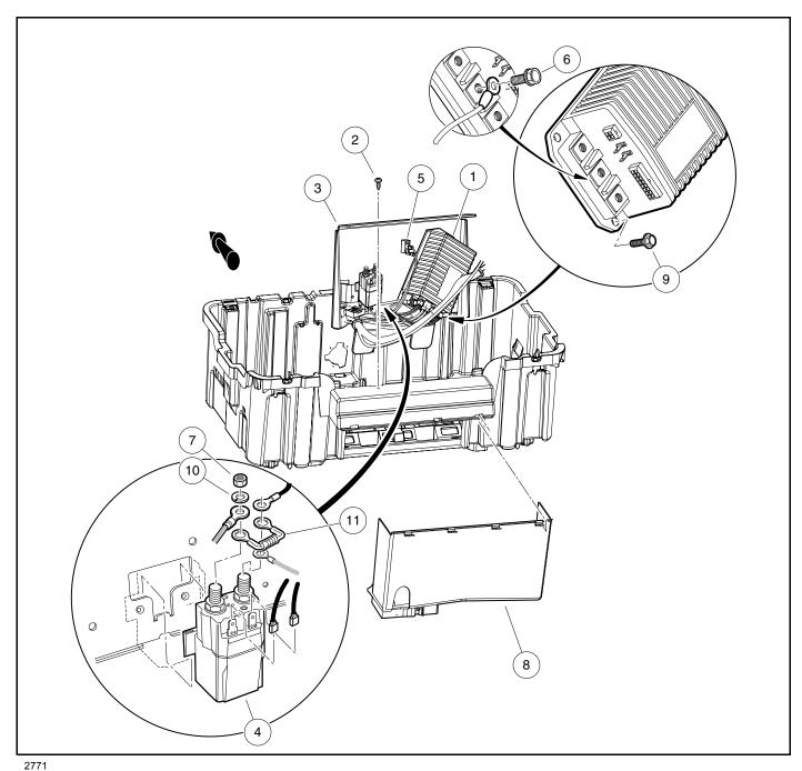
Figure 13-11 Controller and Solenoid Removal
