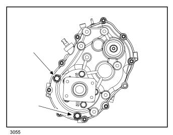
Figure 24-2 Lubricant Level Plug and Drain Plug
