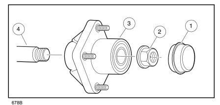
Figure 7-27 Front Wheel Hub Removal
