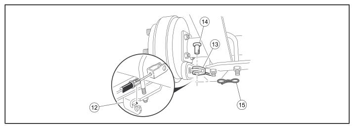
Figure 9-8 Connect Brake Cable
