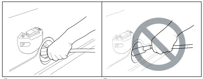
Figure 15-8 Correct Insertion of External Charger DC Plug
