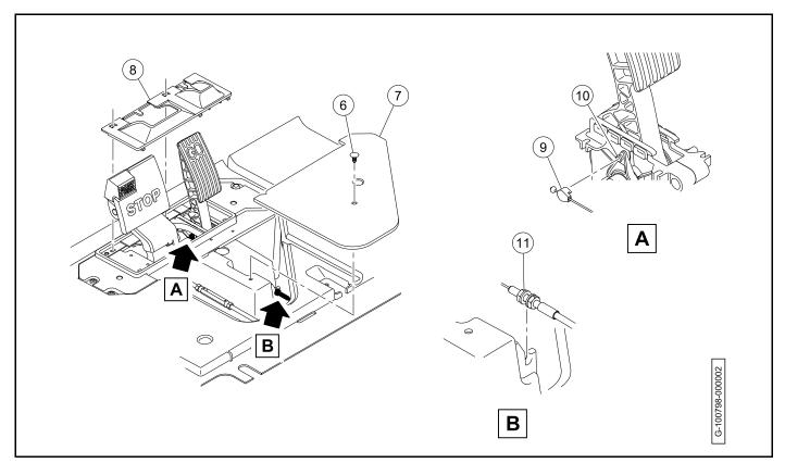
Figure 21-7 Accelerator Cable At Pedal Group
