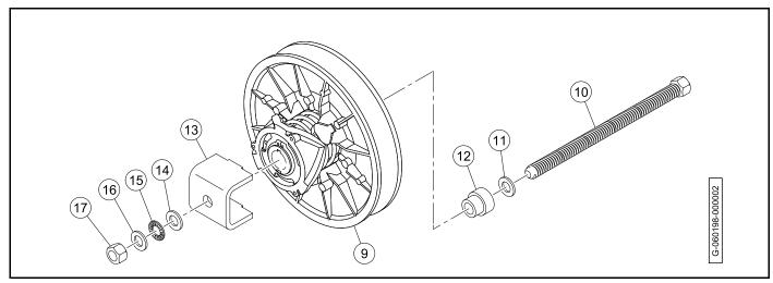
Figure 23-21 Driven Clutch Tool - Assembly
