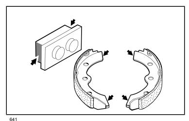
Figure 6-9 Apply Grease To Brake Shoes and Slots
