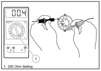
Figure 18-3 Key Switch Test - Engine Kill Circuit
