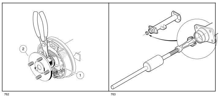
Figure 17-1 Remove Internal Retaining Ring
