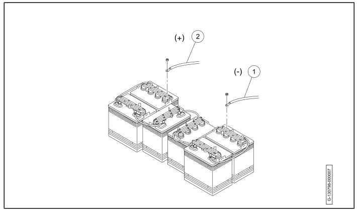
Figure 1-2 Disconnect Electric Vehicle Batteries
