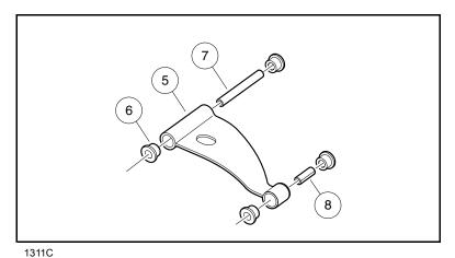
Figure 7-21 Control Arm Removal
