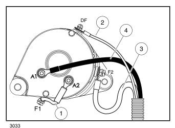
Figure 19-14 Starter/Generator Wiring
