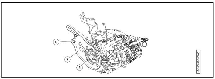
Figure 20-7 Clutch Plate Installation
