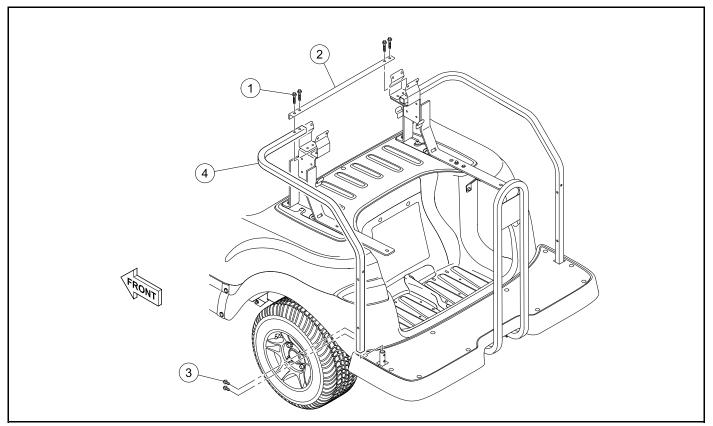
Figure 4-45 Fixed Rear Seat Hip Restraint
