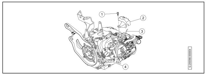
Figure 20-1 Governor Cover and Ground Cable Removal
