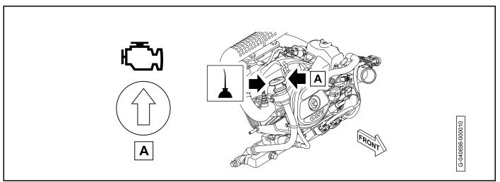
Figure 10-9 Engine Oil Fill Location
