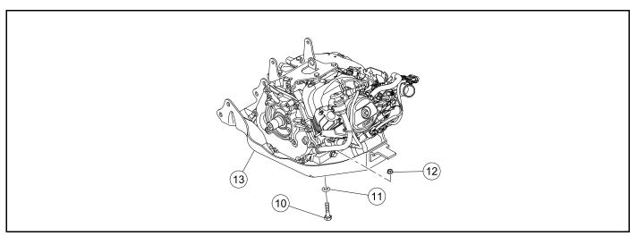
Figure 20-4 Engine Pan Removal
