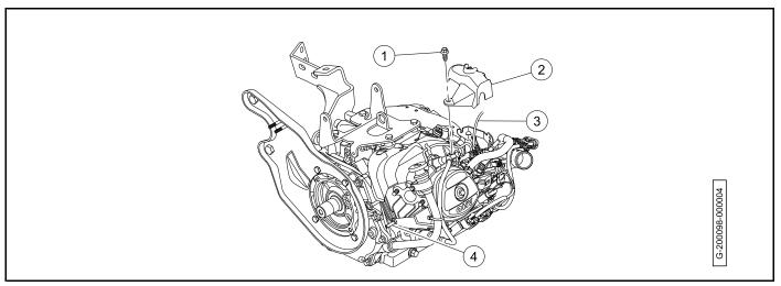
Figure 20-8 Governor Cover and Ground Cable Installation
