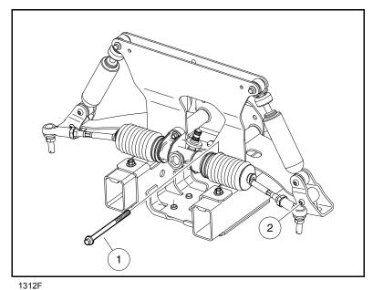
Figure 7-22 Control Arm Bolt Installation
