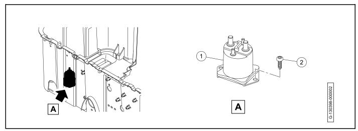
Figure 19-19 Solenoid Installation
