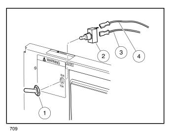
Figure 13-9 Tow/Run Switch
