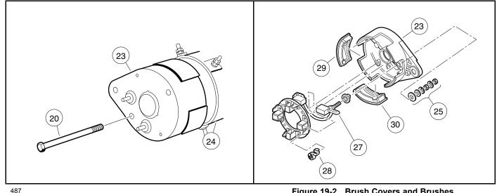
Figure 19-1 Commutator End Cover
