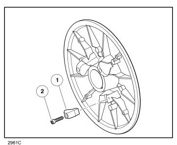
Figure 23-18 Drive Button Inspection
