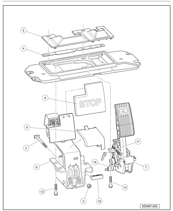
Figure 5-5 Accelerator Pedal Assembly and Brake Pedal Assembly
