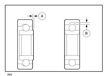
Figure 19-7 Bearing Play Inspection
