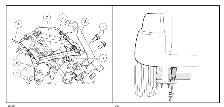
Figure 24-6 Governor Arm, Cable and Brackets
