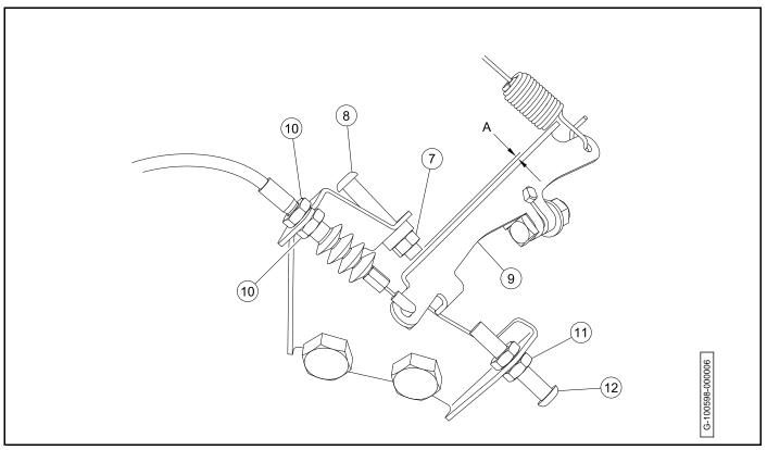
Figure 21-5 Governor Cable Adjustment
