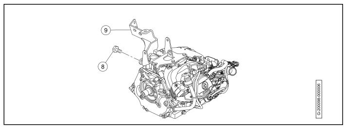
Figure 20-6 Exhaust Weldment Installation
