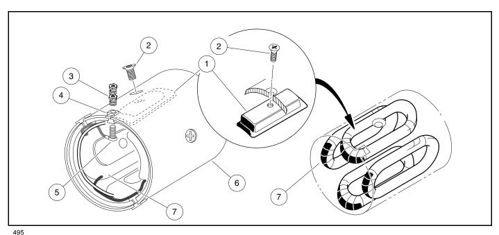
Figure 19-9 Field Coil Assembly
