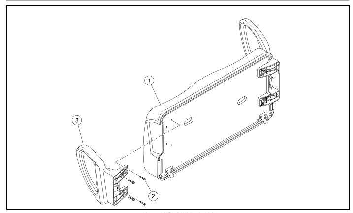
Figure 4-2 Hip Restraint
