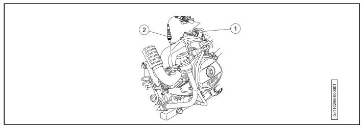
Figure 19-41 Oxygen Sensor
