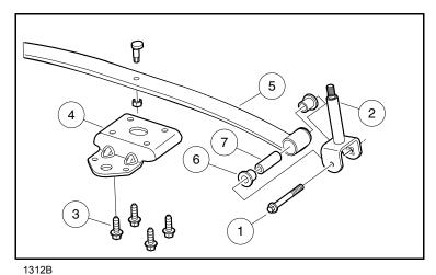
Figure 7-16 Leaf Spring Installation
