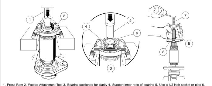
1. Press Ram 2. Wedge Attachment Tool 3. Bearing sectioned for clarity 4. Support inner race of bearing 5. Use a 1/2 inch socket or pipe 6. Press against armature shaft 7. Use bearing puller if a press is not available
