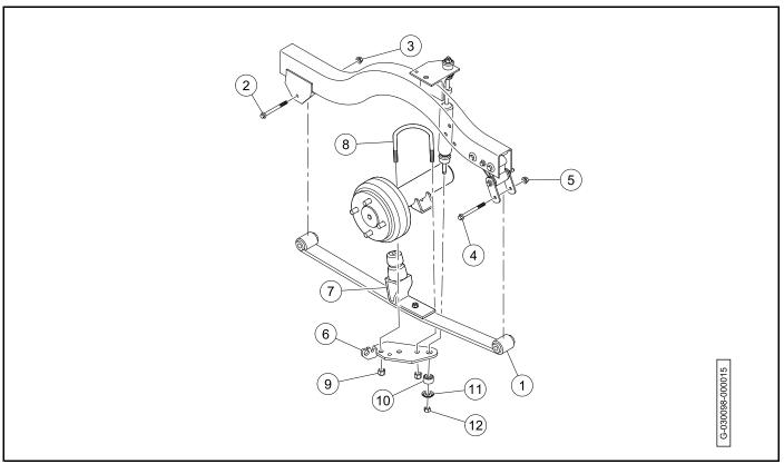
Figure 9-11 Leaf Spring Installation (Four-Passenger)
