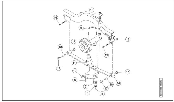
Figure 9-10 Leaf Spring Removal - Four-Passenger
