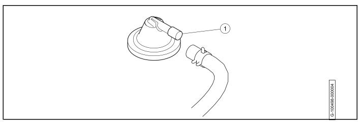
Figure 3-3 Fuel Tank Vent Nipple
