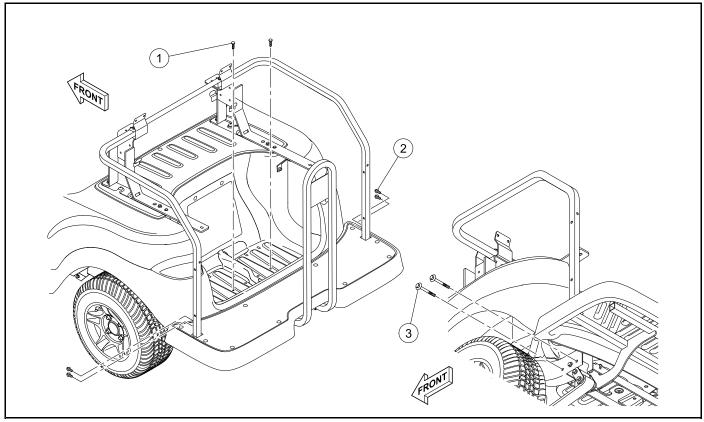
Figure 4-54 Foot Deck (2+2) Installation
