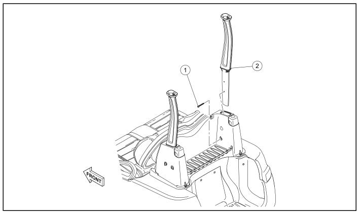
Figure 4-24 Rear Canopy Support Installation
