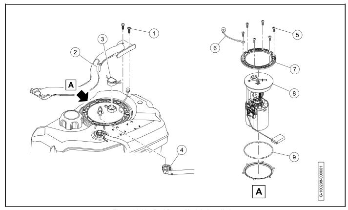
Figure 21-20 Fuel Pump Module Installation
