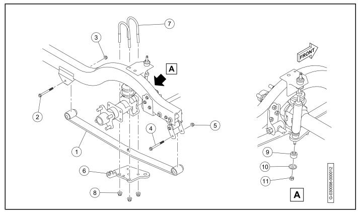
Figure 9-15 Leaf Spring Installation (Four-Passenger - Heavy Duty With Panhard)
