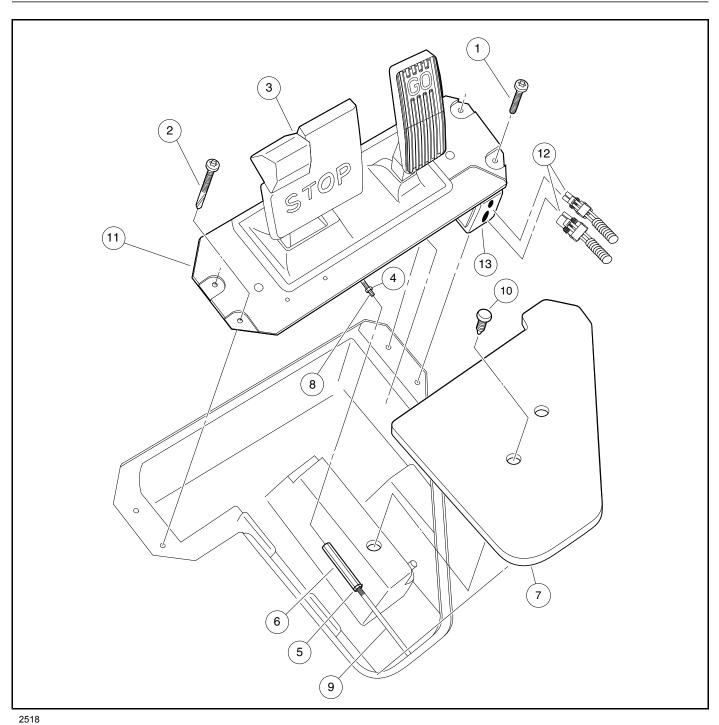
Figure 5-2 Pedal Group - Electric Vehicle
