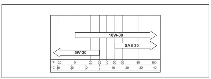
Figure 10-4 Engine Oil Viscosity
