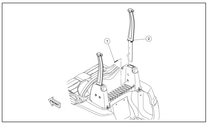
Figure 4-23 Rear Canopy Support Removal
