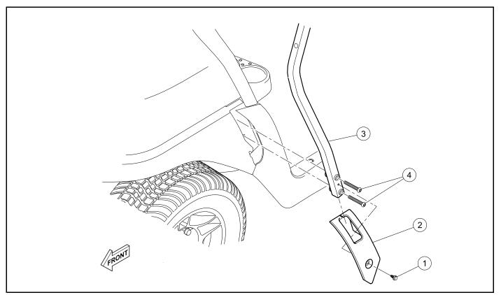
Figure 4-37 Front Canopy Strut Removal
