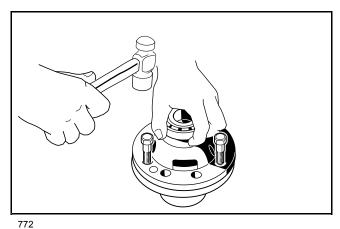
Figure 17-13 Separate Housing
