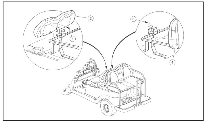
Figure 4-41 Seat Back Removal
