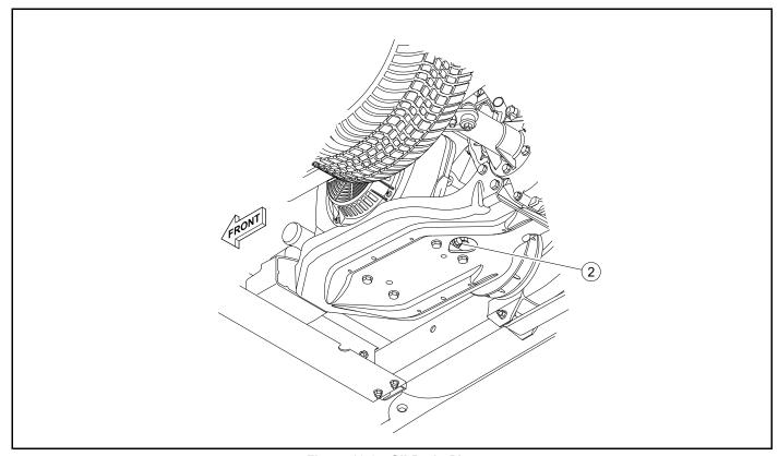
Figure 10-8 Oil Drain Plug
