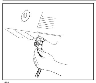
Figure 11-2 Communication Port Under Instrument Panel
