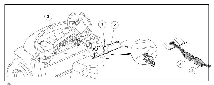
Figure 11-3 Instrument Panel Assembly Removal and CDT Port Connection
