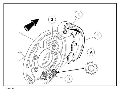
Figure 6-12 Install Adjuster Wheel, Trailing Shoe
