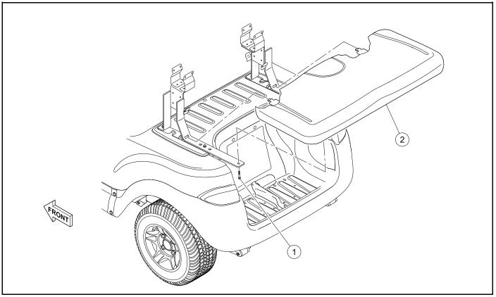
Figure 4-43 Fixed Rear Seat Bottom
