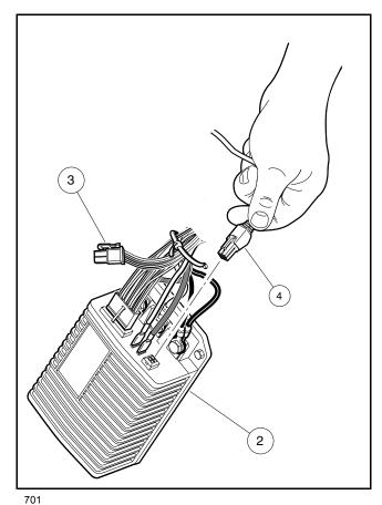
Figure 11-4 CDT Connector On Controller
