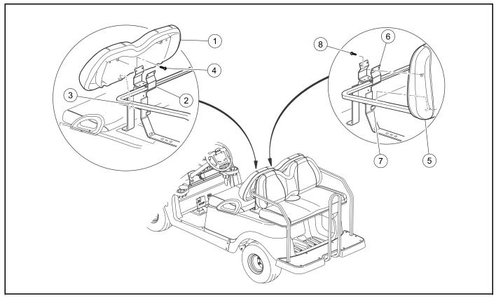
Figure 4-42 Seat Back Installation
