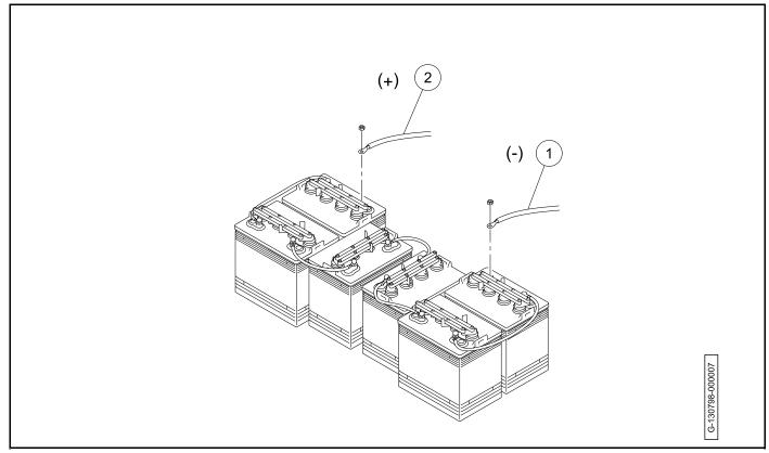
Figure 1-3 Connect Electric Vehicle Batteries
