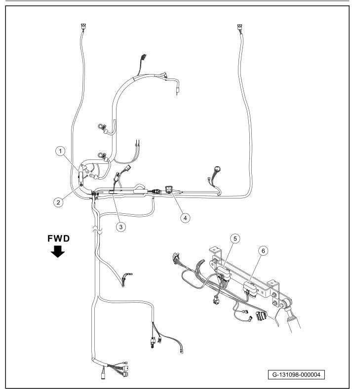
Figure 18-2 Fuse and Relay Locations
