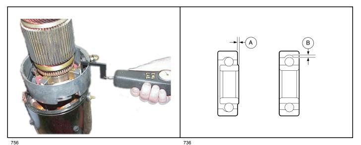
Figure 16-13 Brush Spring Tension Test
