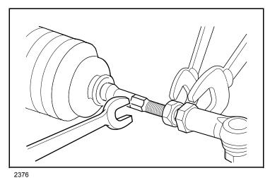
Figure 7-11 Loosen Jam Nuts
