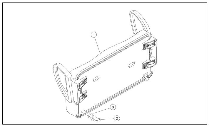
Figure 4-1 Seat Bottom Hinge
