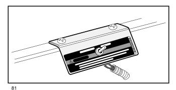
Figure 24-1 MAINTENANCE/OPERATE Switch
