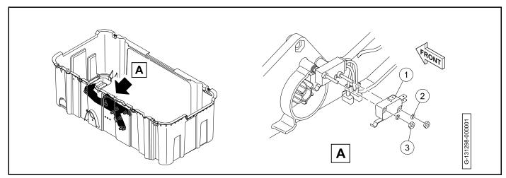
Figure 19-26 Neutral Lockout Limit Switch Removal
