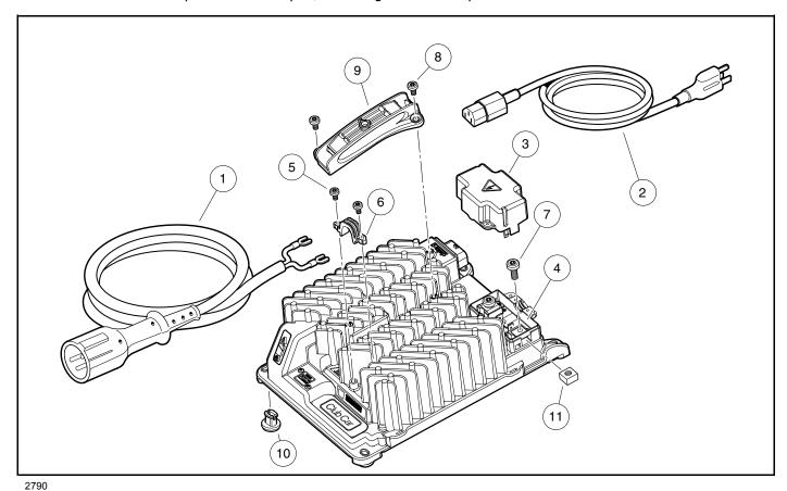
Figure 15-10 External High-Frequency Charger Components
