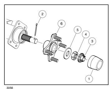
Figure 24-3 Rear Hub Exploded View
