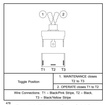
Figure 18-6 Maintenance/Operate Switch Test
