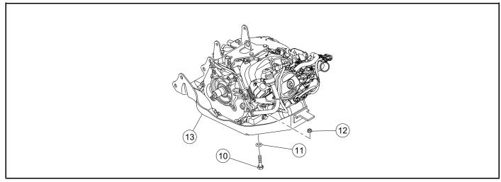
Figure 20-5 Engine Pan Installation
