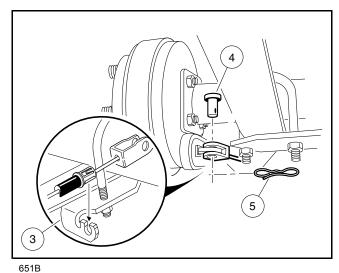
Figure 6-31 Connect Cables at Rear Brakes
