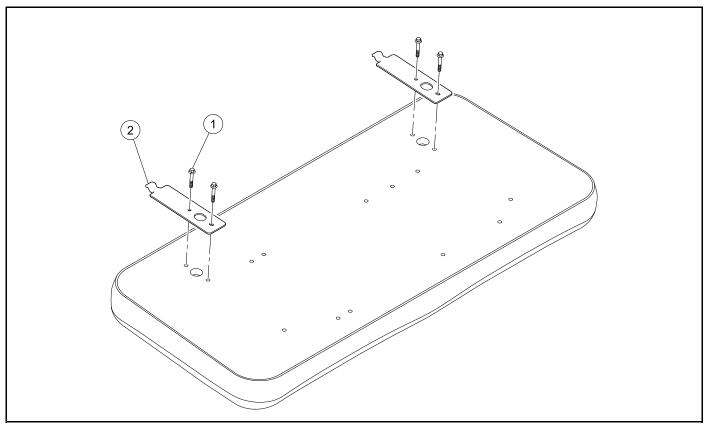
Figure 4-44 Fixed Rear Seat Hinge
