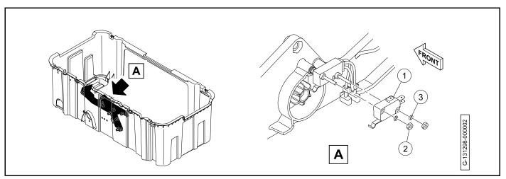
Figure 19-27 Neutral Lockout Limit Switch Installation
