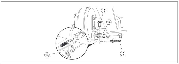
Figure 9-12 Connect Brake Cable
