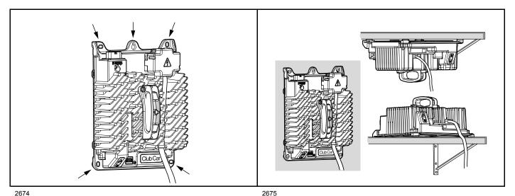
Figure 15-3 Charger Mounting Holes
