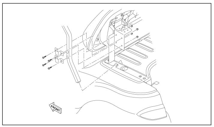
Figure 4-40 Rear Canopy Support Installation
