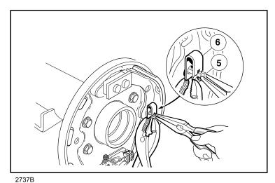
Figure 6-13 Install Trailing Shoe Retainer Clip
