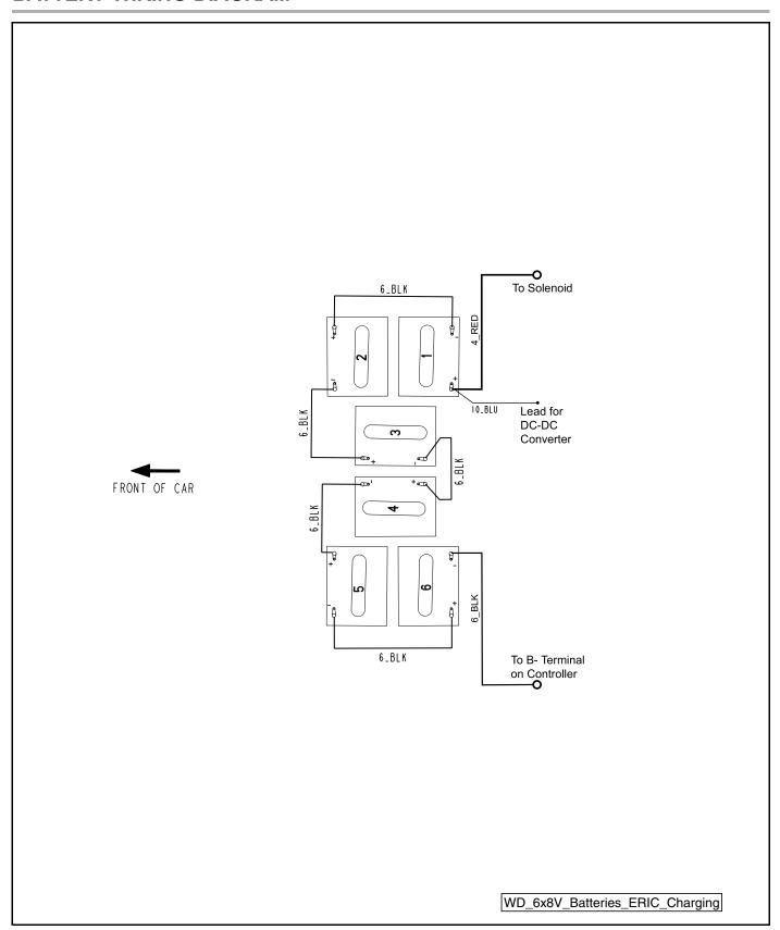
Figure 12-1 Battery Wiring Diagram
