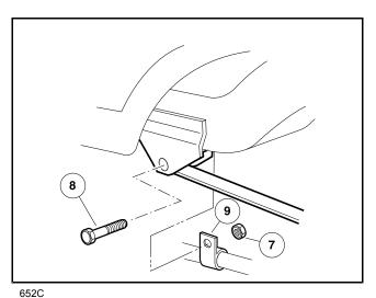
Figure 6-26 Brake Cable Mounting Tab
