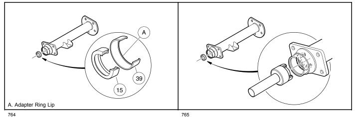
Figure 17-3 Axle Seal and Adapter Ring
