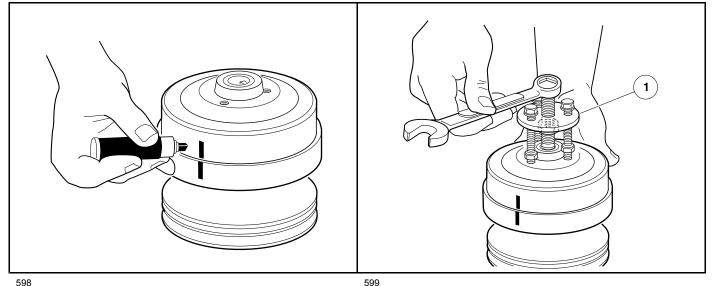
Figure 23-5 Mark Drive Clutch Hub
