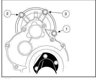
Figure 16-24 EJ8–4001A Motor Mounting Bolts and Tightening Sequence
