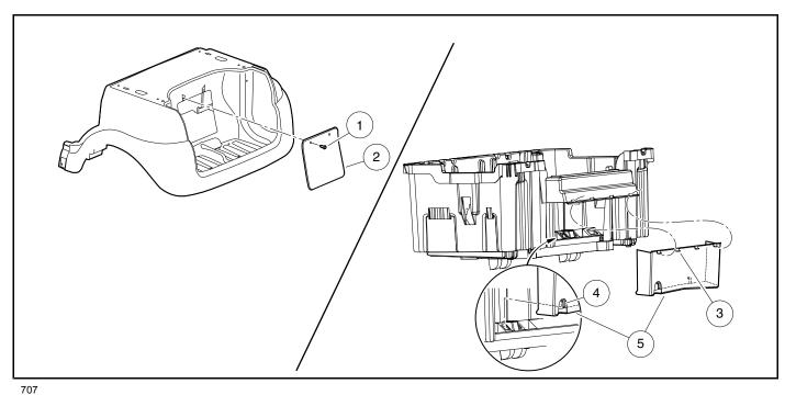
Figure 13-8 Access and Remove Electronics Module Cover
