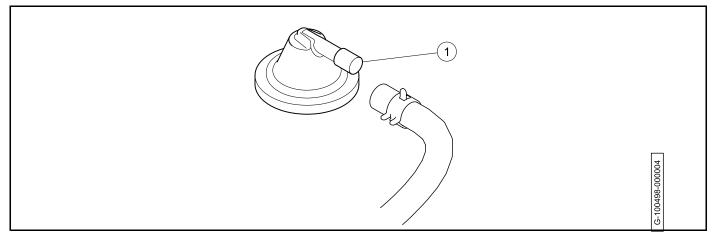
Figure 3-1 Fuel Tank Vent Nipple
