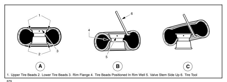
Figure 8-1 Tire Removal
