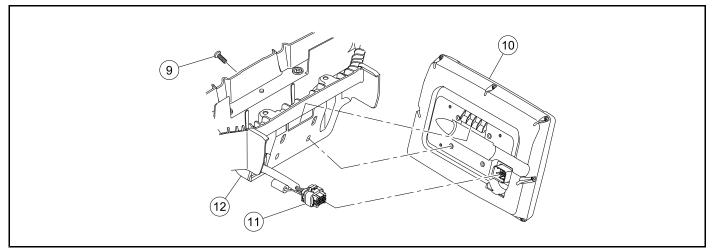
Figure 4-18 Visage Display Unit Removal
