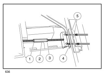
Figure 6-1 Loosen Turnbuckle
