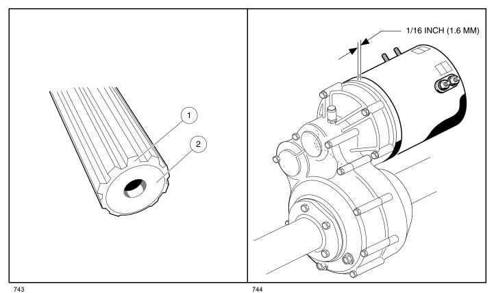
Figure 16-22 Clean Chamfer and Input Shaft End
