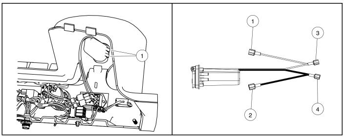
Figure 13-5 USB Port Removal
