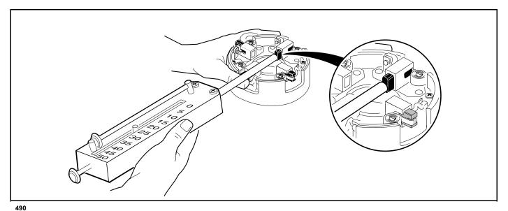
Figure 19-4 Brush Spring Tension Test
