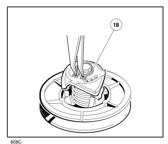
Figure 23-22 Install Retaining Ring
