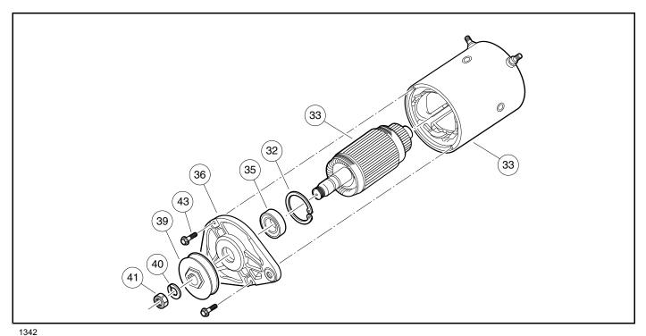
Figure 19-6 Output End Cover Assembly, Armature and Housing
