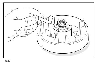
Figure 23-10 Spiral Back-up Rings
