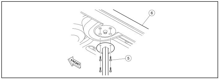
Figure 4-35 Canopy Installation - Rear Canopy Support
