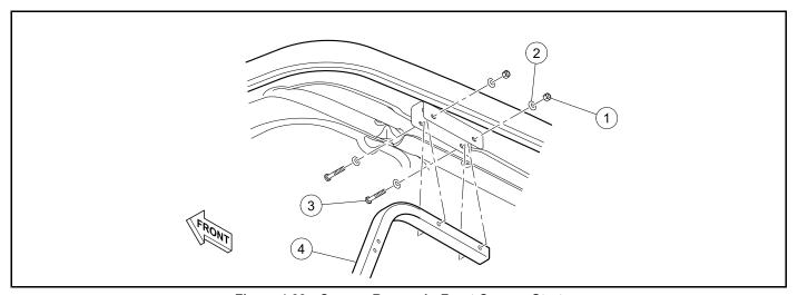
Figure 4-33 Canopy Removal - Front Canopy Strut
