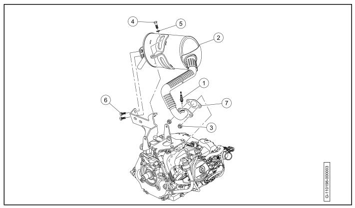
Figure 22-2 Muffler Installation
