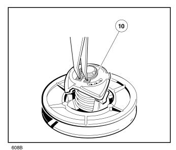
Figure 23-15 Remove Retaining Ring
